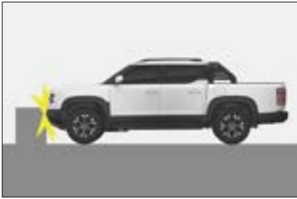
The vehicle's nose hits the ground when going down a steep slope.
